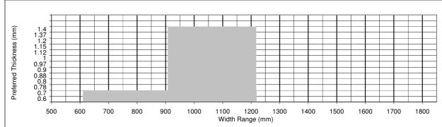
Note: Where maximum widths are less than 1200mm, any width between half maximum and 610mm is available by negotiation only. Availability applies only to dimensional restrictions and is subject to BlueScope Steel Sales and Marketing confirmation. product supplied direct from Western Port and may change if supplied from BlueScope Steel Service Centres. Slitting and shearing available on request from BlueScope Steel Sales Offices.
